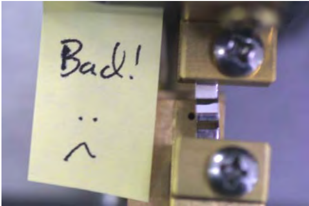
Box filament not centered over air jet & crooked This is BAD!
