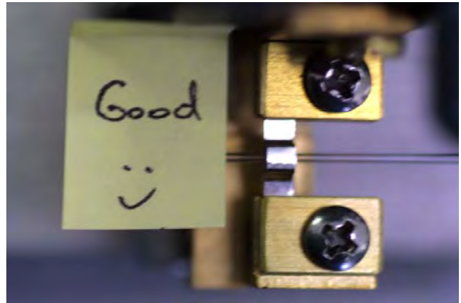
Box filament is centered over the air jet and is 1.0mm in from the left edge of the brass jaws. The filament is positioned so the glass runs through the center of the filament. This is GOOD!
