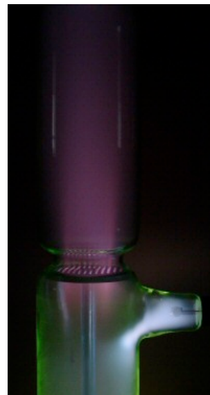
Canal Rays or positive Protons (red glow)
