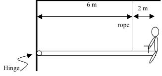
10. Find the tension in the supporting cable and the forces exerted by the hinge in the diagram below if the mass of the beam is 10 kg and the total length of the beam is 10 meters.
