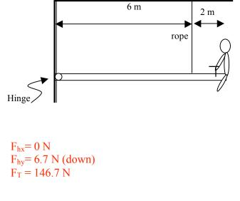
10. Find the tension in the supporting cable and the forces exerted by the hinge in the diagram below if the mass of the beam is 10 kg and the total length of the beam is 10 meters.
