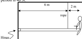
horizontal force of hinge=0 N vertical force of hinge=6 2/3 N up tension=93 1/3 N
