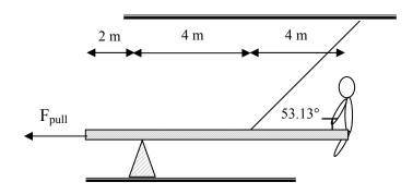
tension=625 N force<sub>pull</sub>=375 N left force of support=0 N
