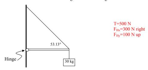
[2] Find the tension in the cable <u>and</u> both the horizontal and vertical components that the hinge supplies to the bar (remember direction).
