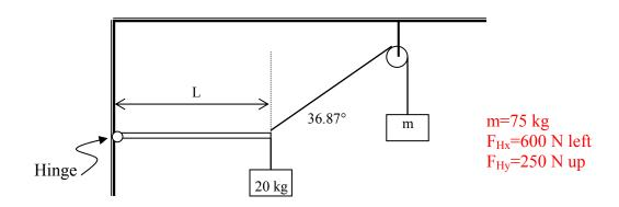
[4] Find the minimum coefficient of friction (µ) required between the end of the bar and the wall in order to maintain static equilibrium.
