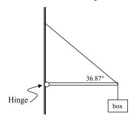
[2] Find the tension in the cable <u>and</u> both the horizontal and vertical components that the hinge supplies to the bar (remember direction). Note: The bar is 60 kg, the box is 60 kg & "L" meters long
