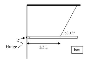
[4] What mass box should be suspended so that the vertical component that the hinge supplies to the bar is zero? Note: The bar is 120 N.
