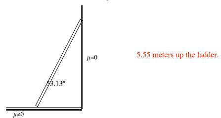
[4] A 10 meter long ladder leans against the wall as shown. If the ladder weighs 200 N and the floor is frictionless, what is the tension in the rope (attached to the middle of the ladder) when a 600 N person stands at the top?
